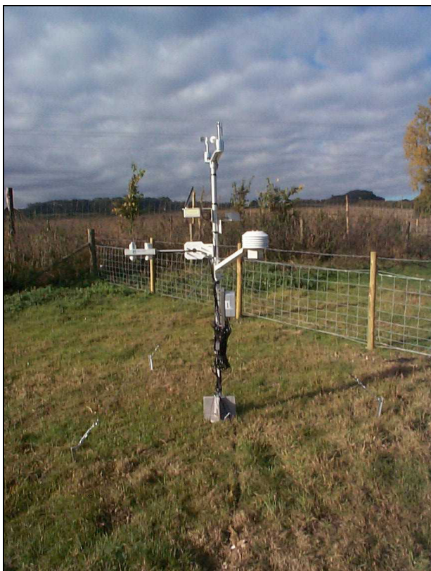
Automatic weather station in the Pang/Lambourn catchments
